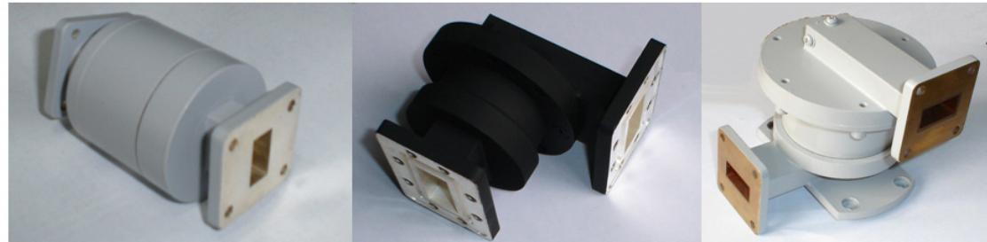
Rotary Joints (rotary couplers) are used to transmit microwave energy from stationary lines to rotating lines. The rotary joint is an electro-mechanical device with RF performance dependent upon rigorous electrical and mechanical design. Available styles are defined by physical geometry as follows:
